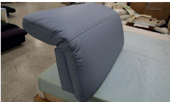
Additional seam in the headboard for leather cutting
